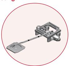
A steering system with a turntable has a minimum weight of 880 kg (including rigid axle). The extra weight means your truck uses more fuel. Moreover, this system is very high maintenance. Just consider all the lubrication points and replacement of the turntable.
